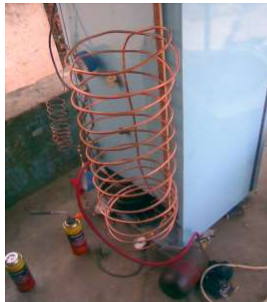
Fig.6 Helical condenser coil diameter of 225 mm
